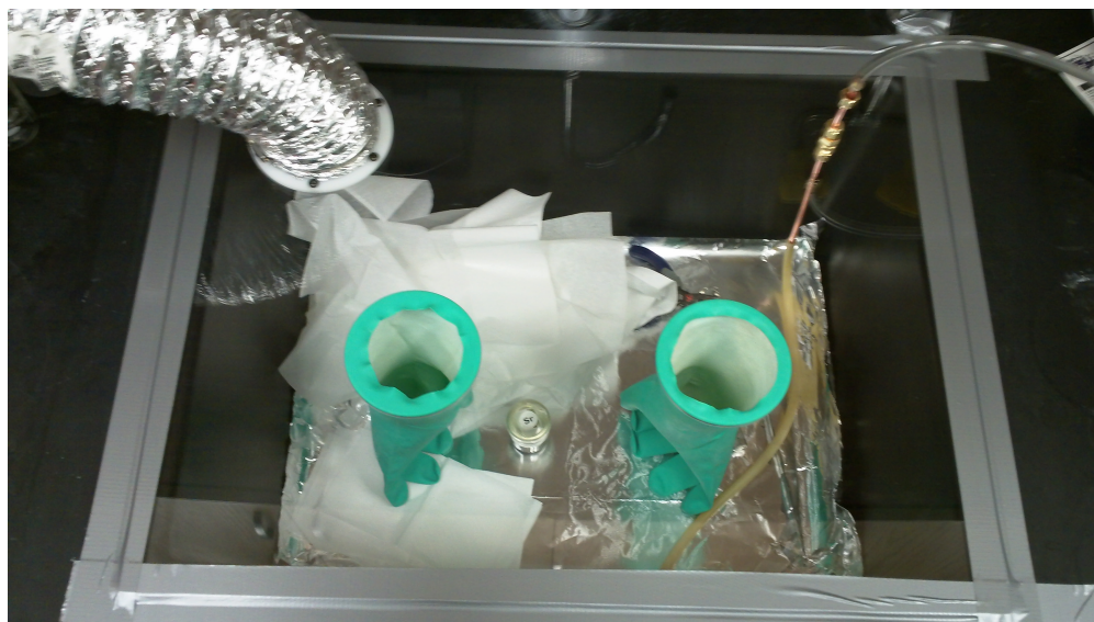
Figure D.2 Picture of the glove box fashioned from the lab sink.
